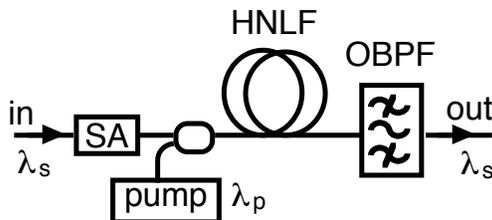
Fig.1. Schematic of a signal regenerator. SA: saturable absorber, HNLF: highly nonlinear fiber, OBPF: optical bandpass filter.
