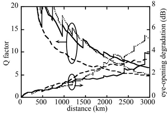
Fig.4. Q factor and EO-degradation versus distance for 40Gb/s quasi-linear transmission.
