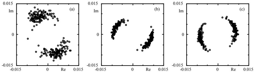
Fig.5. Distribution of amplitude and phase at pulse peaks at 2960km. (a) No regenerators are inserted, (b) regenerators are inserted every 6 spans, and (c) regenerators are inserted every 3 spans.
