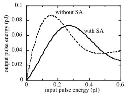
Fig.2. Energy transfer function of the FWM regenerator with and without saturable absorber.
