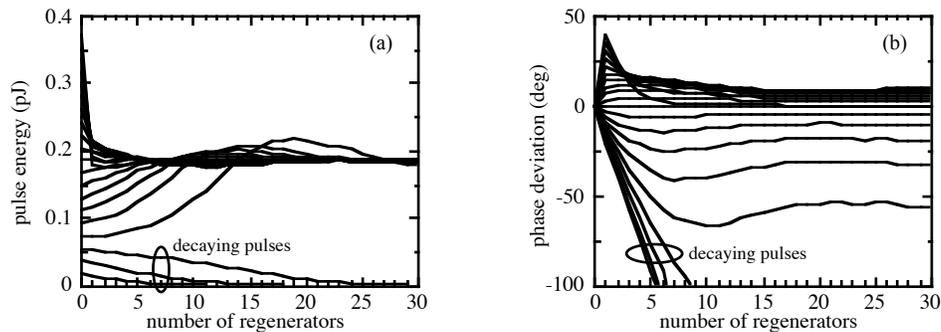
Fig.3. Evolution of pulse energy (a) and phase at pulse peak (b) in cascaded regenerators. Initial pulse amplitude is varied among 20 different values. Gain of the amplifier between regenerators is fixed at 3.2.
