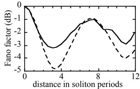
Fig.2. Noise reduction by temporal modulation (solid curve) or by spectral filtering (dashed curve).
