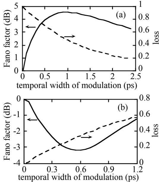
Fig.1. Noise enhancement and reduction by temporal modulation. (a) Gaussian modulation function  $m_1(t)$  and (b) Inverse-Gaussian (notch) modulation function  $m_2(t)$  are applied.
